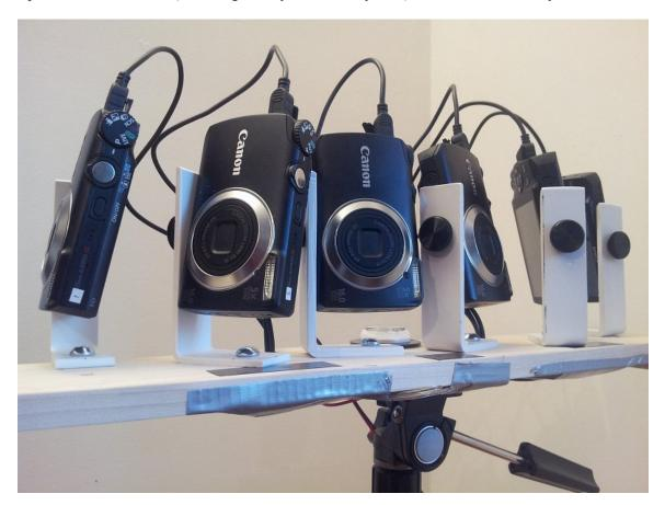
Sounds too good to be true, right? Well, there is a catch. The 96 megapixel "camera" is actually an array of six 16 megapixel cameras. And, there is some assembly required! These six cameras are triggered to shoot at exactly the same moment, with each camera capturing a different portion of the scene. The images produced by
