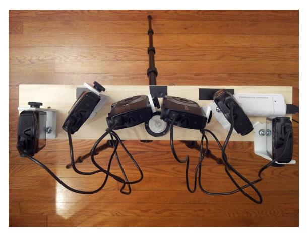
The board measures about 18 x 3.5 inches, and weighs a little less than a pound. With all of the cameras, cables and other hardware attached, the total weight is about 3 pounds, about a pound lighter than a Nikon D800 DSLR and Nikon 14-24 lens. Because the array is quite light, it doesn't require a particularly sturdy tripod. I have been using mine with a small Slik Compact XL tripod.
